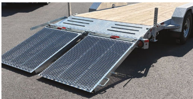
Split gate ramps with springs (8,500 lb capacity)
