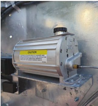
E-SERIES Electro-hydraulic brake (1,200 psi)
