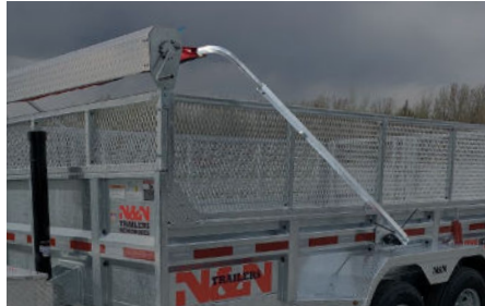
Aluminum spring-assisted tarp
