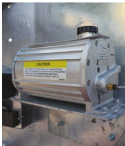
E-SERIES Electro-hydraulic brake (1,200 psi)
