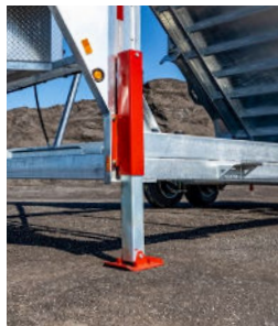
H-SERIES Front hydraulic jack 12,000 lb capacity
